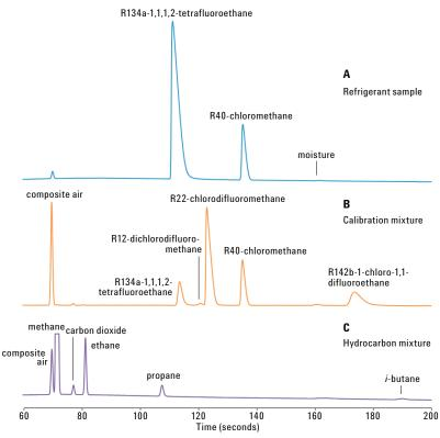
Figure 1. Speed-of-analysis - The Agilent 490 Micro GC delivers fast characterization of the refrigerant mixture.
