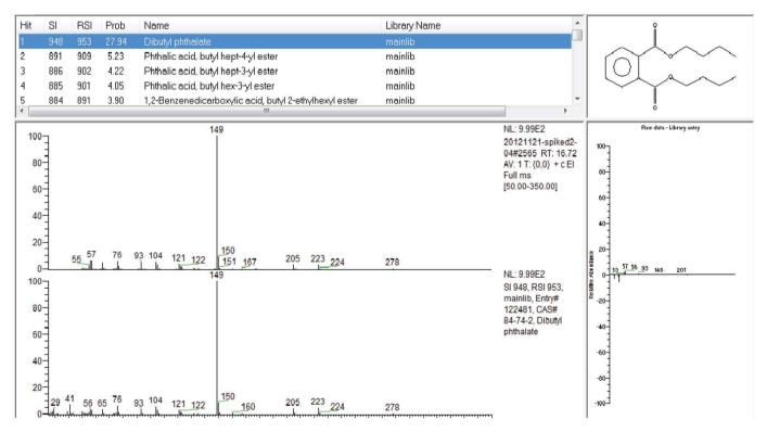
Figure 8. Comparison of spectra between the spiked sample (top) and NIST library (bottom) indicating excellent spectral match value. Similarity Index = SI, Reversed Search Index = RSI
