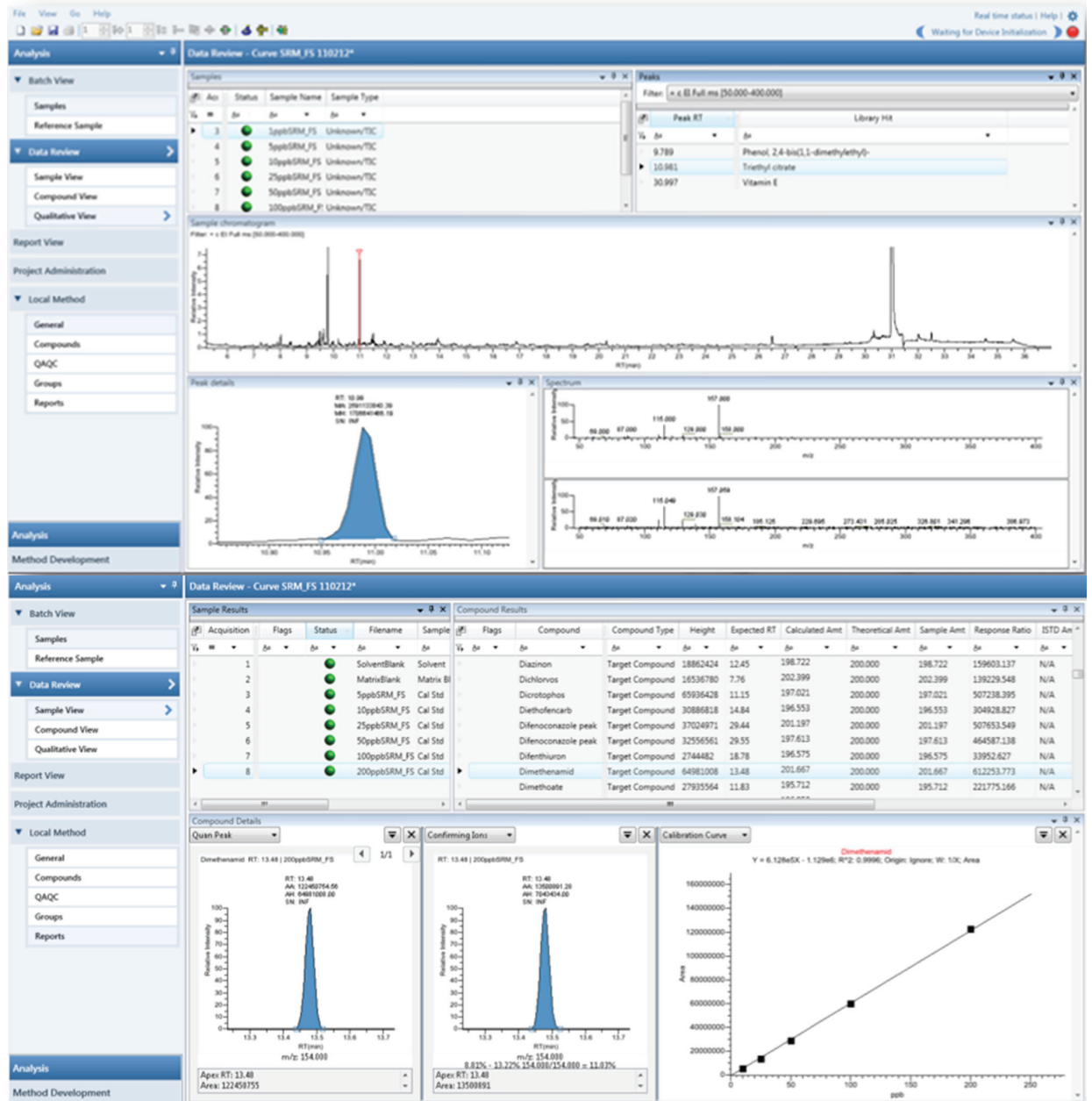
Figure 7. Qualitative view of TraceFinder EFS software for analyzing fruit juice with simultaneous full scan/ Timed-SRM on the TSQ 8000 system. In addition to quantitating and confirming the 158 target compounds by MRM (top), TraceFinder EFS software has identified three high-level unknowns by full scan analysis (bottom): 2,4-bis(1,1-dimethylethyl)-phenol, triethyl citrate, and Vitamin E.
