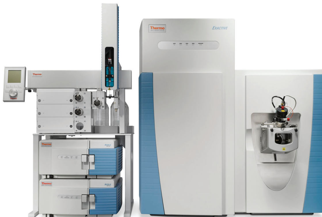
Figure 1. EQuan MAX system equipped with the Exactive mass spectrometer and ExactFinder software
