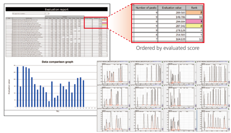
Ordered by evaluated score A browser also allows for visual evaluation of multiple chromatograms.
