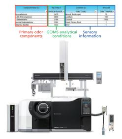
Since some odor components have a low odor threshold, low concentration levels need to be detected to identify the causative substances. High-sensitivity MRM/SIM analysis by GC-MS(/MS) can reliably detect even trace components near the odor threshold (a few pg/g).
