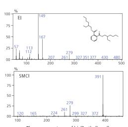
The mass spectrum of bis(2-ethylhexyl) phthalate (MW=390) obtained using different ionization methods
