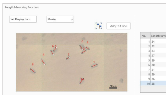
Fig. 5 Length Measurement Operation Screen and Measurement Length Results
