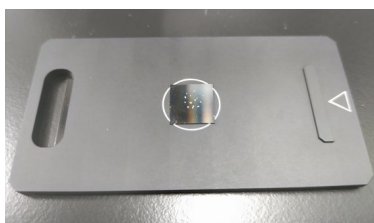
Fig. 1 Si Filter Installed in the PF Holder
