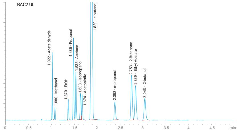
FID chromatogram of Agilent's Blood Alcohol Checkout mix (p/n 5190-9765) demonstrating transfer and resolution of all 12 components. The sample was prepared by combining 50  $\mu\text{L}$  of the mix with 450  $\mu\text{L}$  of 0.1% (v/v) t-butanol in water in a 20 mL headspace vial.
