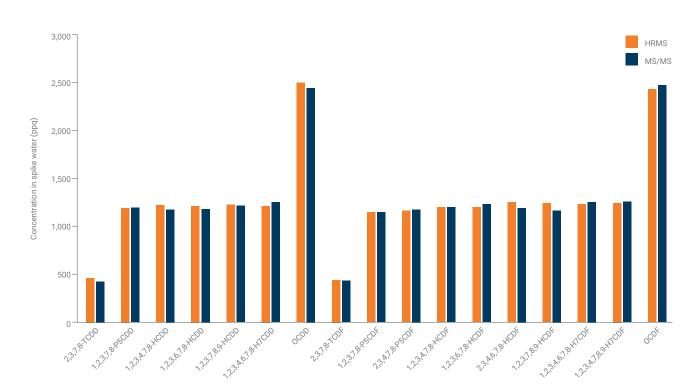
Comparable results were achieved when comparing the concentration determined by GC/HRMS and GC/MS/MS analysis of a spiked water sample.
