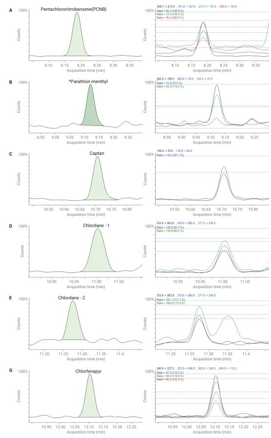
A) PCNB at 0.0625 ppb; B) methyl parathion at 0.016 ppb; C) captan at 1.00 ppb; D) chlordane-1 at 0.25 ppb; E) chlordane-2 at 0.25 ppb; G) chlorfenapyr at 0.25 ppb
