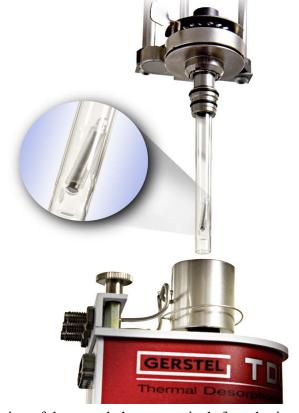
**Figure 1.** The GERSTEL Twister, used for stir bar sorptive extraction of drugs and pharmaceuticals from brain tissue in the work reported here.
