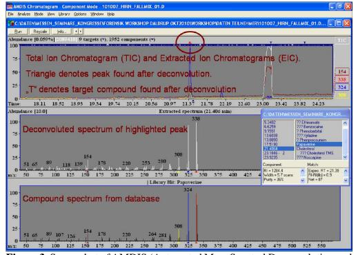
**Figure 3.** Screenshot of AMDIS (Automated Mass Spectral Deconvolution and Identification System) software.
