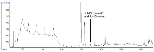
Figure 1: SIM Scan of a 2ppb Standard with the Static HT3 Headspace Parameters. The retention times of 1,4-dioxane and 1,4-dioxane-d8 are located on the chromatogram.
