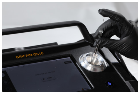
Fig 4 Direct syringe injection performed on Griffin G510
