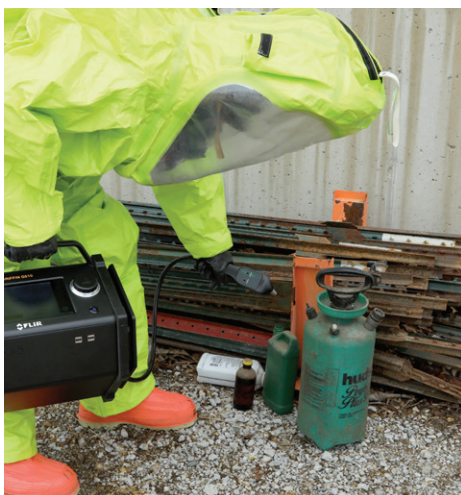
Fig.3 The Griffin G510 can be operated while wearing full PPE
