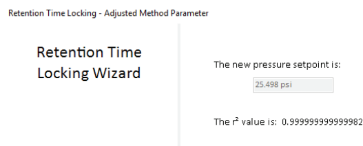
Figure 7. Retention time locking pressure calibration results.
