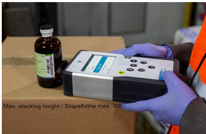
Figure 1. The Agilent Vaya Raman handheld spectrometer with SORS being used to identify materials through an amber bottle in a warehouse.
