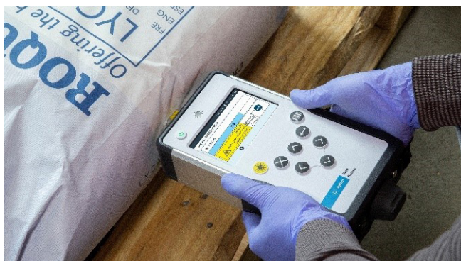
Figure 1. The Agilent Vaya Raman handheld spectrometer being used to identify materials inside sacks in a warehouse.
