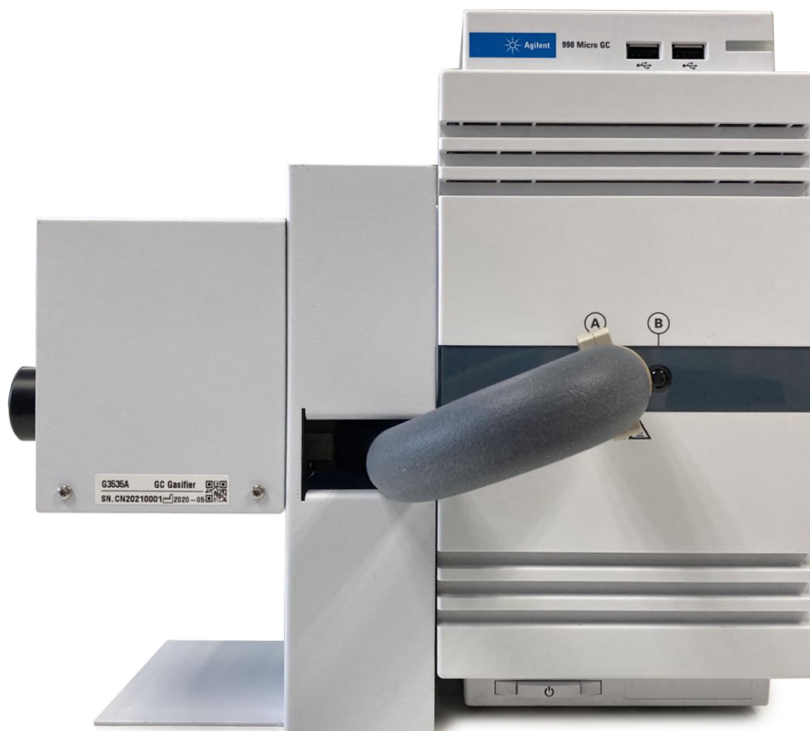
Figure 1. The Agilent G3535A GC gasifier installed on the Agilent 990 Micro GC.
