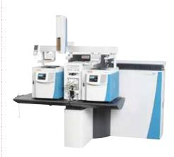
Unique double-GC configuration for maximum flexibility. For example PCDD/F on GC one and PCBs on GC two.
