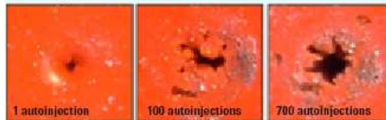
High-Temperature Septa Without CenterGuide: Major Coring Before 100 Autoinjections
