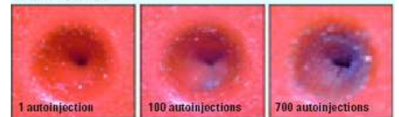
Agilent BTO Septa With CenterGuide: Very Little Coring Even After 700 Autoinjections
