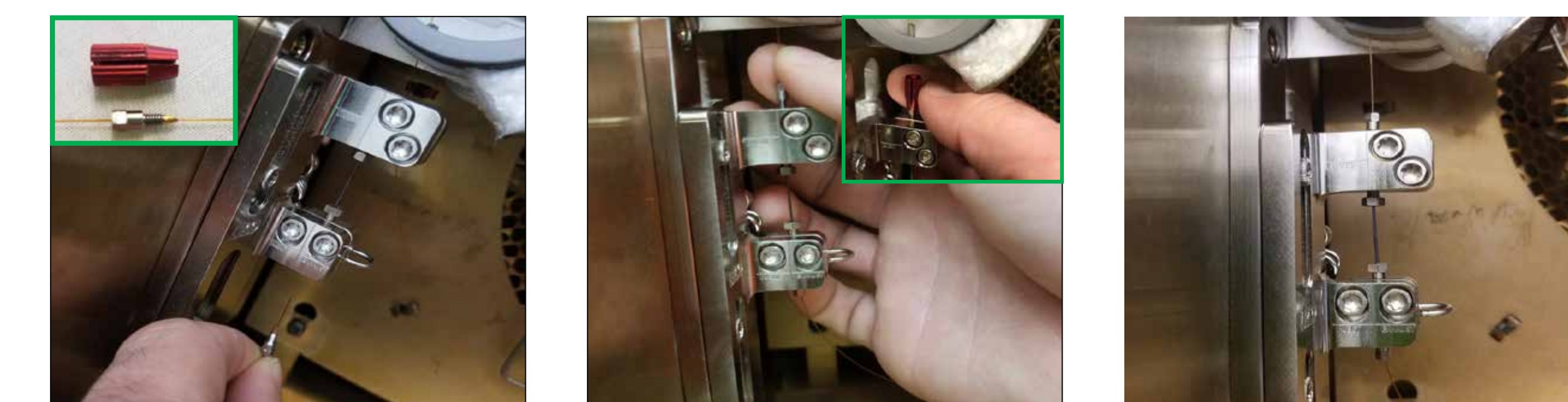
Figure 5. The installation of the columns procedure into the FLUX modulator. (Left) The primary column inserts through the bottom of the modulator until it comes to a hard stop. The captured nut (upper left inset) and ferrule is tightened using the provided hand tool (upper left inset). (Middle) The secondary column threads down through the top of the modulator until it encounters a hard stop, and like the primary column the nut with ferrule is tightened using the hand tool to provide a robust leak-free connection. (Right) The system is assembled and ready to run.
