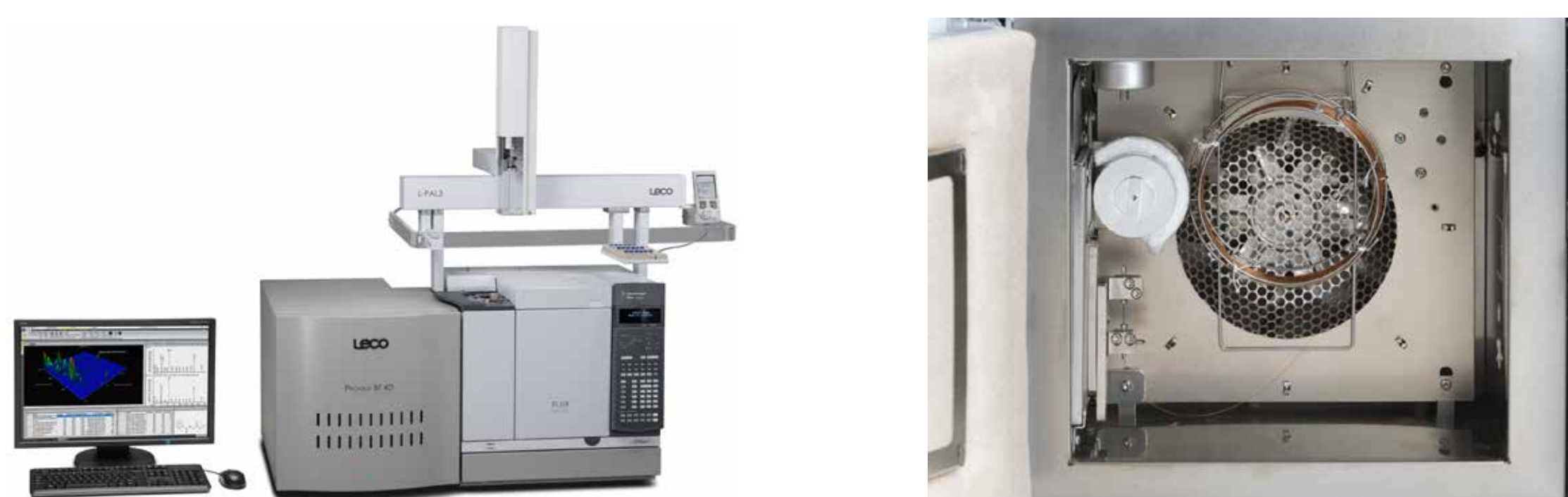
Figure 1. (Left) Pegasus BT 4D with FLUX flow modulator; (Right) The inside of the GC oven with the FLUX modulator.
