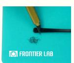
Precision Scissors Cut quartz wools protruding from sample cup (Eco-cup).
