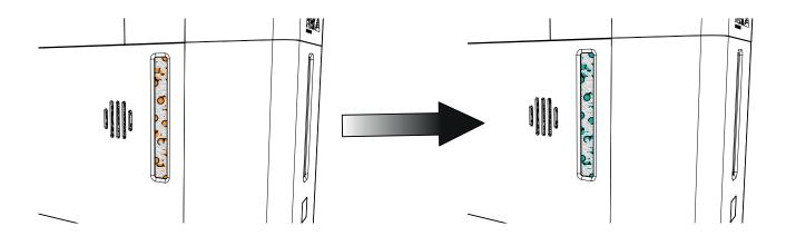
1. To replace the capsule, **depressurise the generator and disconnect power.** Lift the hinged lid back, then unscrew the capsule cap anticlockwise to remove.
