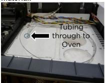
4. Once the stainless steel tubing has been pushed through and secured, the end of the tubing should be aimed at the inlet of the GC column.
