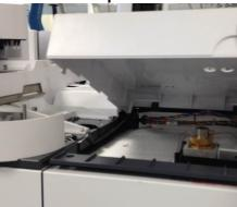
2. Locate the cut-out hole on the aluminium plate directly above the rear hole on the GC oven.
