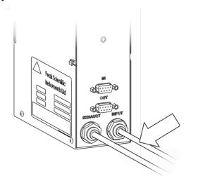
Fit the 1.5m of  $\frac{1}{4}$ " OD  $\frac{x^3}{_{16}}$ " THK tubing provided to the detector's **EXHAUST** port. It is recommended that this is then connected to a fume hood or other extraction device.
