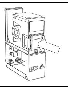
With the cover removed, the cartridge (06-9006) can now be fitted to the detector. Ensure that there is no protective cover over the sensor head and that the side clips are unclipped by pulling outwards.
