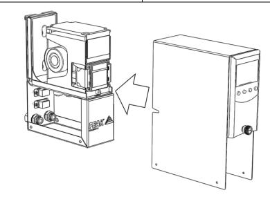
The cover can now be refitted, Ensuring that the thumbscrew and the 4 hex screws are securely fastened.
