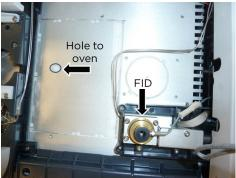
3. Make a hole through the insulation material, through to the oven. The stainless steel tubing from the detector can now be pushed through the hole, and secured in place using more insulation material.
