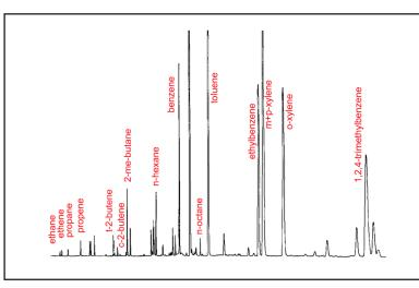
Extended HC analysis on FID (emission gas sample; He or  $\rm H_{2}$  carrier gas)
