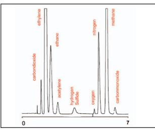
Channel 2: permanent gases on TCD (He carrier gas)
