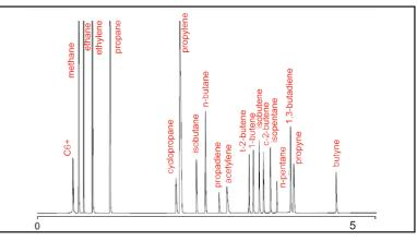
Channel 3: C1-C6 hydrocarbons on FID (He or H<sub>2</sub> carrier gas)
