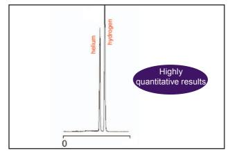
Channel 1: helium / hydrogen on TCD (N<sub>2</sub> carrier gas)
