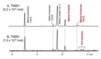
Fig. 1: Pyrograms of soybean oil with varied amounts of TMSH Py temp.: 350°C, Oven temp.: 40 – 240°C(20°C/min), Column: UA-CW (polyethylene glycol) (L=30 M, i.d.=0.25 mm, df=0.25 µm), Carrier gas He: 1 mL/min, split ratio: 1/50
