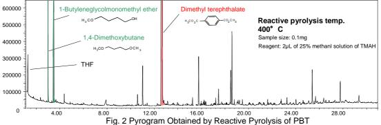
Carrier gas: He, Injection port pressure: 103kPa, Split ratio: 1/60, Separation column: Ultra ALLOY\*-5 (5% diphenyldimethylpolysiloxane)
