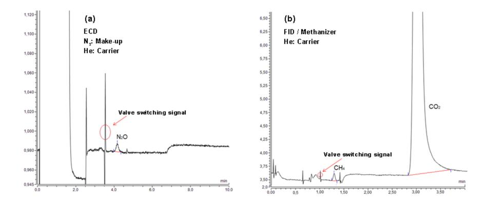
32.76 ppb of N<sub>2</sub>O detected by ECD; (b) 0.056 ppm of CH<sub>4</sub> and 7.432 ppm of CO<sub>2</sub> detected by FID/Methanizer
