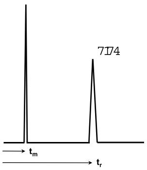
$t'_r = tr - tm$  $t'_r = 4.41 - 1.25$  $t'_r = 3.16$  min = time spent in stationary phase
