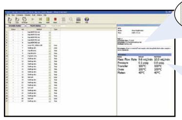
Schedule Screen - The autosampler scheduling screen allows for multiple method and technique types within one schedule. This feature allows the user to run both static and dynamic methods as well as M.O.M. methods all in the same sequence without having to change any hardware. In addition the use of vial inserts allows for 9 mL, 12 mL and standard 22 mL vials to be varied within the sequence as well.
