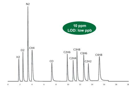
Chromatogram 1: permanent gases and light hydrocarbons, 10 ppm level
