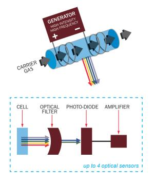
Diagram 1: Plasma Emission Detector, principle
