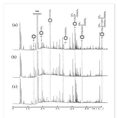
Fig. 1 Pyrograms of PMMA samples obtained at 460°C
