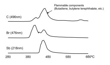
**Fig. 2** Thermal decomposition of flame retardant PBT observed by evolved gas analysis (EGA)
