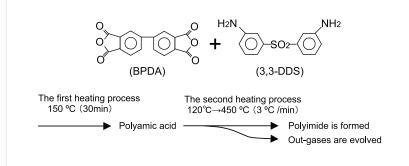
Fig. 1 The synthetic process of polyimide
