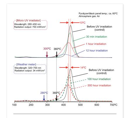
**Fig. 1** Thermograms obtained before and after irradiation by UV/Py-GC/MS (top) and Xe weather meter (bottom). Pyrolyzer temp.: 100 - 700°C (20°C/min), GC oven temp.: 300°C, UADTM-2.5N (L=2.5 m, i.d. =0.15 mm), Carrier gas flow rate: 1 mL/min; He, split ratio: 1/50, sample: 20ug
