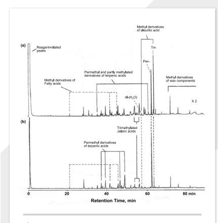
Fig. 1 Typical pyrograms of Indian Shellac obtained at 400°C (a) In the absence of TMAH, (b) In the presence of TMAH solution
