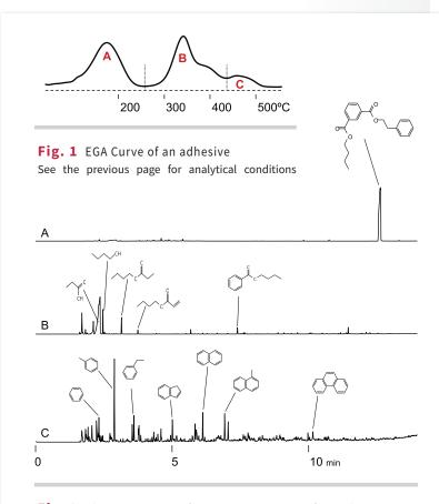
**Fig. 2** Chromatograms of temperature zones of EGA thermogram Pyrolysis temp.: 40°C~600°C (20°C/min), Column flow rate: 1ml/min, Split ratio: 1/50 Separation column: Ultra ALLOY+-5 (5% diphenyl polysiloxane), 30m, 0.25mm id, df=0.25μm GC oven temp.: 40°C~320°C (20°C/min), Sample: 0.8mg, Detector: MS (m/z=29-400, 2scans/sec
