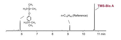
Fig. 1 Chromatogram of TMS-derivatized PC sample obtained by TD-GC/MS
