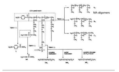
**Scheme 1** Formation pathway of typical products of UV-cured resin after reactive pyrolysis
