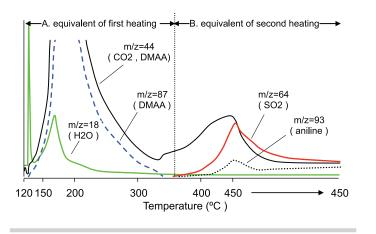
**Fig. 2** Thermogram with mass chromatogram in the process of polyimide synthesis
