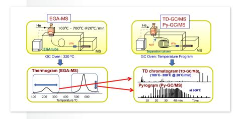
Following EGA, the instrument is re-configured. The EGA tube is replaced by an analytical column. The Frontier Vent-Free Adaptor enables this to be done easily and quickly; there is no need to vent the MS. MS vacuum equilibrium is re-established within a few minutes, and the exposure of the ion source to oxygen is minimized.
