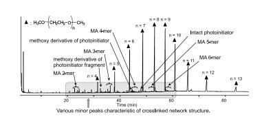
**Fig. 1** Typical pyrogram of UV-cured resin prepared from polyethyleneglycol diacrylate and morpholino-type photo-initiator. Pyrolysis temp.: 400°C, GC oven temp.: 35°C (6 min)-(5 °C/min)-340°C Separation column: Poly(5% diphenyldimethylsiloxane), L=30 m, id=0.25 mm, df=0.25 μm
