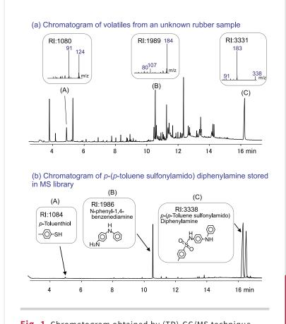
Fig. 1 Chromatogram obtained by (TD)-GC/MS technique
