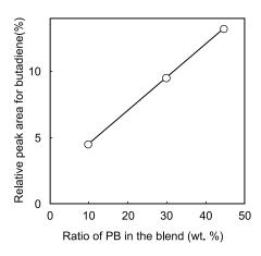
Fig. 2 Calibration curve for PB in the blend
