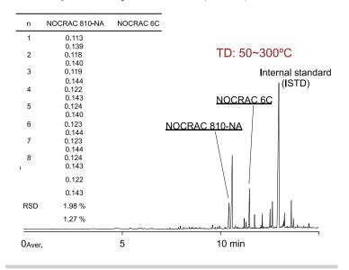
Fig. 2 Chromatogram for Zone A by (TD)-GC/MS analysis
