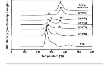
Fig. 1 EGA thermograms of chitin derivative/PVA blend samples obtained by EGA-MS
