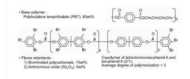
Fig. 1 . Base polymer and structure of flame retardant
