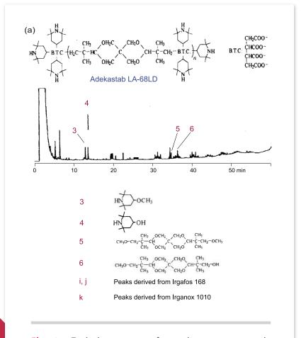
**Fig. 1** Typical pyrogram of a polypropyrene sample obtained by RTD-GC
