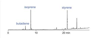
Fig. 1 Fig. 1. Pyrogram of a blend rubber
