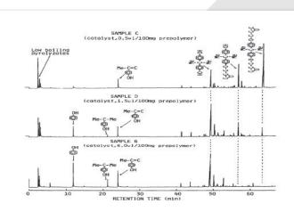
Fig. 1 High-resolution pyrograms of epoxy resins cured with various amounts of imidazole catalyst at 180°C for 3h.
