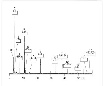
**Fig. 1** Pyrogram of copolyacetal by reactive pyrolysis Pyrolysis temp.; 400°C, GC oven temp.: 50°C-(5°C/min)-300°C, Carrier gas flow rate: 50 ml/min, Separation column: poly(methylphenylsiloxane) L=50 m, id=0.25 mm, di= 0.25 um, Column flow rate: 1.0 ml/min
