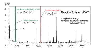
**Fig. 2** Pyrogram obtained by reactive pyrolysis of PBT Carrier gas: He, Injection port pressure: 103kPa, Split ratio: 1/60, Separation column: Ultra ALLOY+-5 (5% diphenyldimethylpolysiloxane) L=30m, Id=0.25mm, df=0.25μm, GC oven temp: 38°C~300°C (20°C /min)
