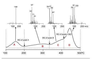
**Fig. 1** EGA curve of ceramic composite material (Injection molding)
