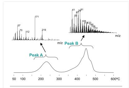
**Fig. 1** EGA thermogram of a rubber and averaged Mass Spectra Furnace temp.:50~600°C (10°C/min), Carrier gas: He 60ml/min, Split ratio:ca.1/50 EGA tube: id=0.15 mm, L=2.5 m (UADTM-2.5N), GC oven temp.: 300°C Sample:ca. 0.5 mg, MS scan range: m/z=29-400, Scan speed: 0.1 scans/sec PY-GC interface temp.: 320°C (AUTO mode)
