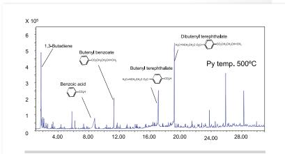
Fig. 1 Pyrogram obtained by flash pyrolysis of PBT
