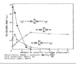
Fig. 2 Changes of characteristic products from epoxy resins as a function of catalyst amount.
