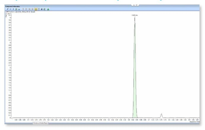
Analysis of 100 fg of OFN: Signal to Noise >7000:1
