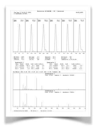
CHROMTECH Evolution3 QqQ Autotune report being generated and automatically printed with a single push of a button in GCMS MassHunter Acquisition software.
