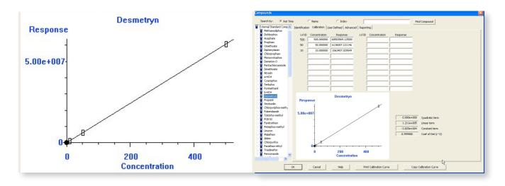
Calibration plot showing excellent linearity over a broad concentration range from 10 to 100 ppb for Desmetryn in Agilent MSD ChemStation Data Analysis software
