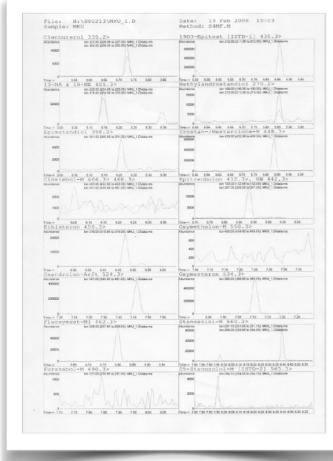
Agilent MSD ChemStation Data Analysis custom report used for analysis of banned substances or its metabolites in urine.
