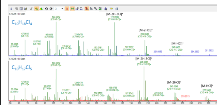
Figure 3. Examples of fragment formula annotated low energy EI spectra for the C 10 Cl 4 and C 10 Cl 5 congeners using 22 eV ionization.
