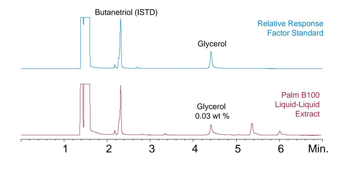
Deactivated stainless steel tubing and Capillary Flow Technology unions are used to connect the external column to the system's split/splitless inlet and FID. This provides an inert flow path for the analysis of polar compounds. This is demonstrated by the analysis of free glycerol extracted from biodiesel.
