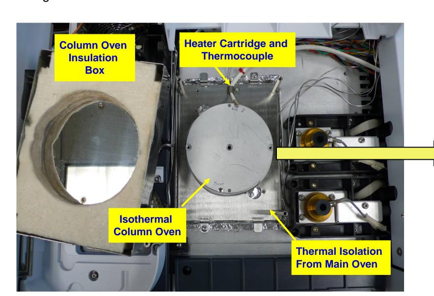
This photo shows the isothermal oven mounted on the 7890A. The oven insulation box is removed and shown on the left. The external oven is thermally isolated from the main column oven using specially designed insulation. A heater cartridge and thermocouple automatically controls the external oven temperature.
