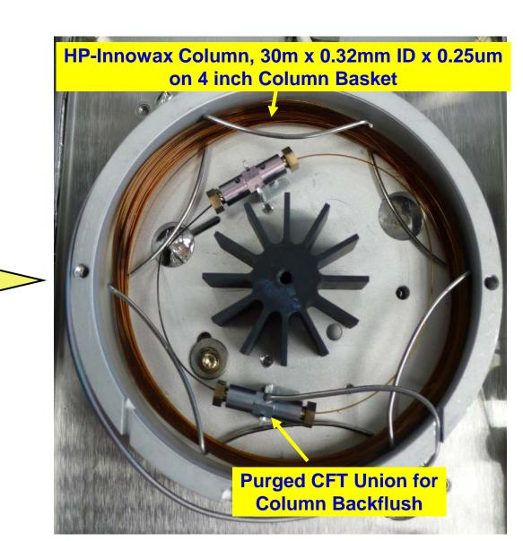
This photo shows the interior of the isothermal column oven. A 4-inch cage contains the 30 m x 0.25 mm ID x 0.25 um capillary column. A Capillary Flow Technology (CFT) union connects the column to the split/splitless inlet via deactivated stainless steel tubing. The column outlet is connected to the FID using a purged CFT inlet. The purged inlet enables the use of backflushing to improve column performance and extend column life.
