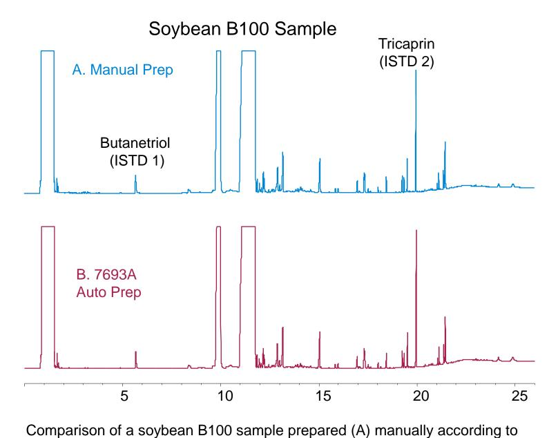
the ASTM D6584 protocol and (B) the 10% scaled automatic protocol using the 7693A ALS.
