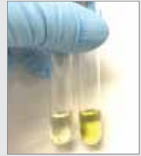
Oasis PRiME HLB clean-up (left) and no clean-up (right).
