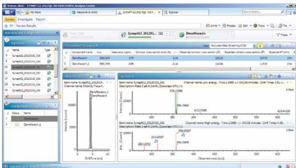
Figure 8. Identification of two danofloxacin protomers identified in porcine extract, where ion mobility resolution spectral cleanup has been selected. Precursor and fragmentation ions with matrix background ions removed, are shown for the danofloxacin protomer with expected CCS 124.70 Å².
