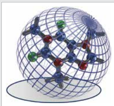
Figure 1. Illustration of rotating three-dimensional conformation of an ion and average collision cross section (shadow).
