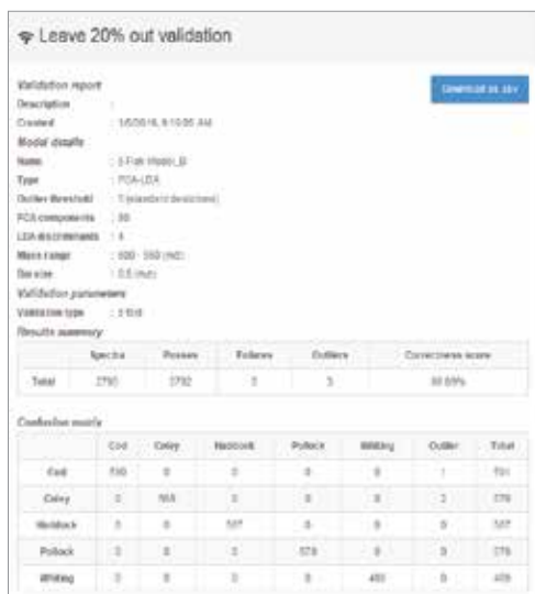
Figure 3. Cross validation (leave 20% out method) results for the REIMS fish model created from 2795 spectra obtained from 478 biological samples (8-12 replicate measurements) of authentic fish. An overall correctness score of 99.89% was obtained with only 1 replicate of cod and 2 replicates of coley classifying as outliers.
