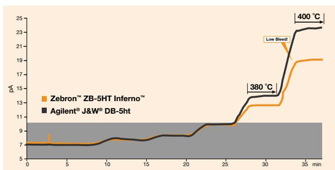
**Figure 2.** Bleed comparison of the DB-5ht and ZB-5HT Inferno. The shaded area depicts the bleed criteria for MS certified columns on a MS detector. MS bleed certification values are typically read at 320 °C. The ZB-5HT demonstrated lower bleed than the DB-5ht. It meets MS certification limits, even at 360 °C.
