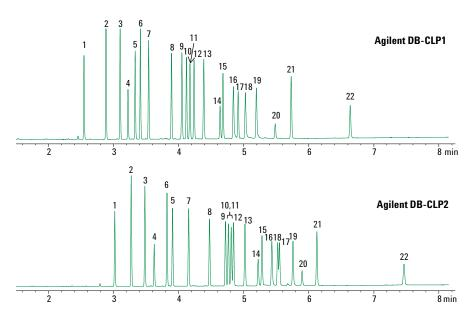
Figure 1. CLP pesticides analyzed on Agilent J&W DB-CLP1 and DB-CLP2 columns.
