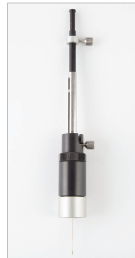
Figure 12: Injection Guide with GC-Specific Adaptor Cup
