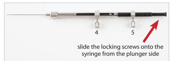
Figure 4: Attaching the Locking Screws to the Syringe
