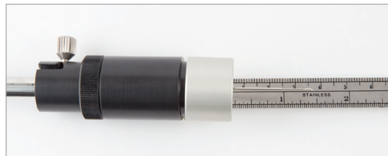
Figure 14: Adjusting the Desorption Depth
