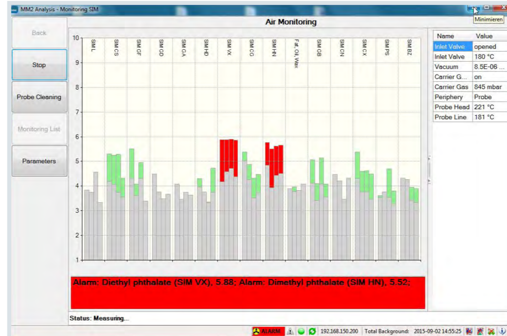
This air monitoring measurement has detected and identified two separate substances simultaneously.
