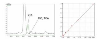
Fig. 3: Left - Mass Trace of SIM ions 195 and 215 (internal Std) of a standard sample of 0.7 ppt TCA. Right- Calibration curve of the 2,4,6,TCA with d-TCA as an internal standard. Concentration range: 0.54 to 53.8 ppt.
