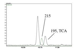
Fig 4: SIM <sup>1)</sup> data recorded with a real cork sample. The determined concentration of 2,4,6 TCA is 6 ppt.
