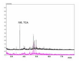
Fig 5: Trace of mass 195 of a fast GCMS full scan data recoded with a red wine spiked with 5 ppt 2,4,6 TCA. The bottom data is relative to a blank wine
