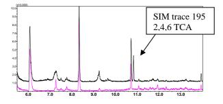
Fig. 2: Top: SIM <sup>1)</sup> data of mass trace 195 relative to an extract spiked with 17 ppt TCA compared with an unspiked extract.
