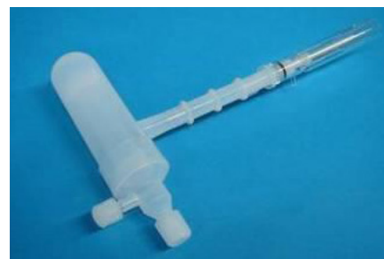
Figure 10. Inert (HF resistant) O-ring-free PFA sample introduction system.
