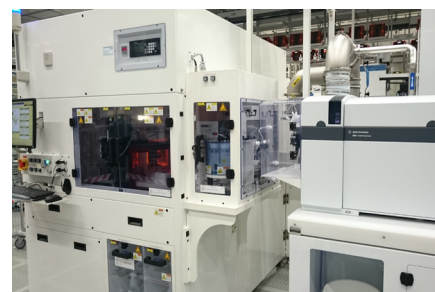
Figure 7. A fully automated VPD-ICP-MS system Expert PS manufactured by IAS Inc., integrated with an Agilent ICP-QQQ. Image provided courtesy of ST Microelectronics, Crolles, France.
