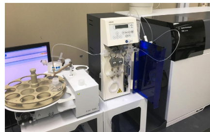
Figure 13. The ASAS automated standard addition device, part of the CSI online monitoring system from IAS Inc., Japan.
