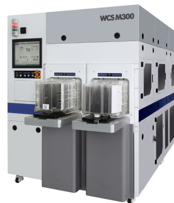
Figure 5. The WCS M300 automated VPD scanner system from NvisANA, Korea.
