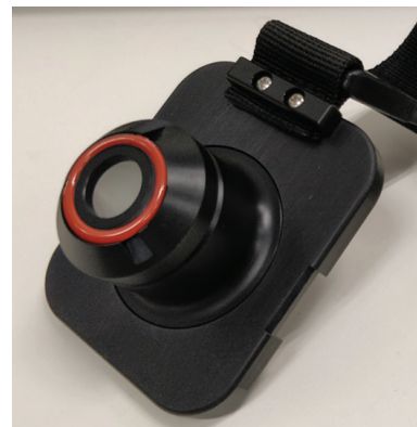
Figure 2. Left: the 45° specular reflectance interface with nonmarking clear fluorinated ethylene propylene (FEP) coated orange silicone O-ring. Right: schematic showing the principles of the technique, often referred to as infrared reflection-absorption spectroscopy (IRRAS); S=Source and D=Detector.
