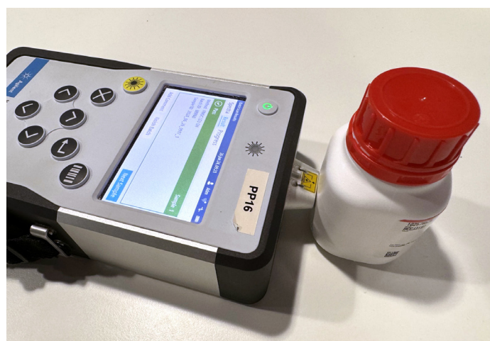
Figure 1. The Agilent Vaya Raman raw material identity verification system being used to verify Fmoc-protected amino acids.
