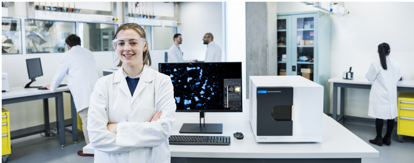
Figure 1. The Agilent 8700 LDIR chemical imaging system allows the high-speed routine analysis of microplastics, including the number of particles present in the sample, their size, and chemical composition.
