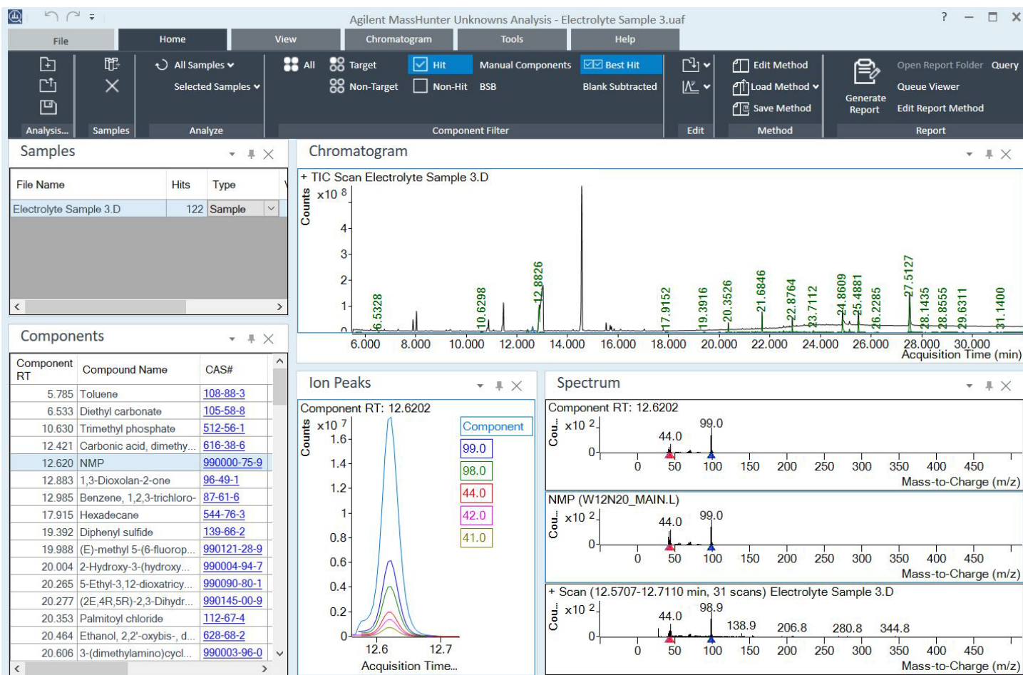
Figure 3. MassHunter unknowns analysis for electrolyte sample 3.
