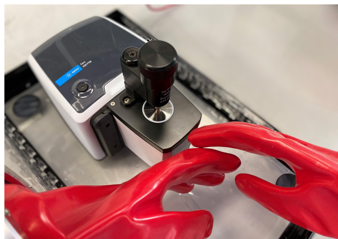
Figure 1. The Agilent Cary 630 FTIR spectrometer with its ultracompact, lightweight design (20 × 20 cm and 3.6 kg) can easily be used in a glovebox to produce high-quality results for moisture-sensitive or hazardous chemicals.
