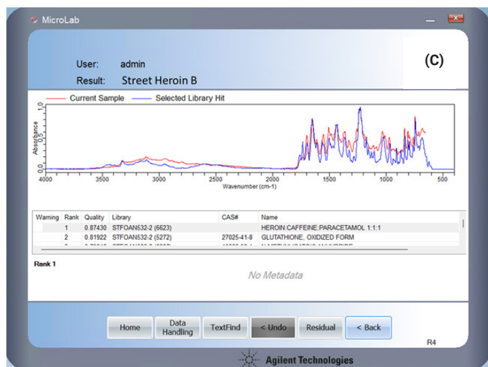
Figure 6. Agilent MicroLab PC software view for a library search of a street sample of heroin (sample B), where the primary identified compound is a 1:1:1 weight ratio of heroin, caffeine, and paracetamol. Displayed are (A) heroin sample B FTIR ATR spectrum; (B) ranked library search results; and (C) Details screen displaying the visual spectral match. Note: residual analysis is not required in this case with the ternary mixture directly identified.
