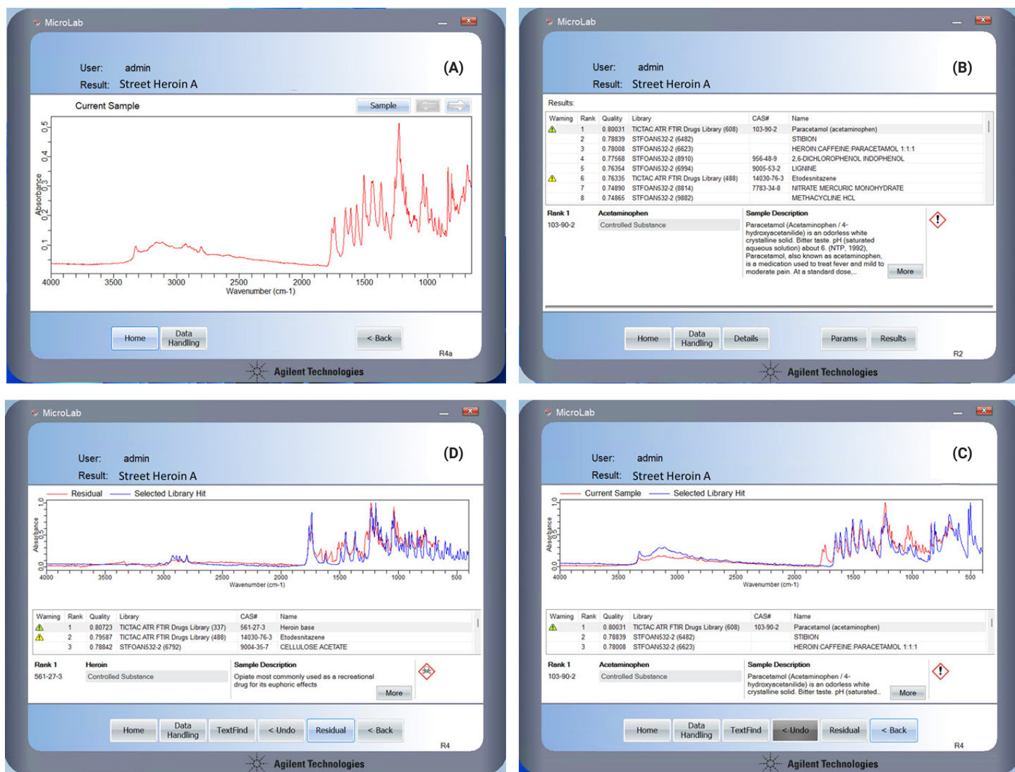
Figure 5. Agilent MicroLab PC software view for a library search of a street sample of heroin (sample A) cut with paracetamol. Displayed are: (A) heroin sample A FTIR ATR spectrum; (B) ranked library search results for the primary identified compound—paracetamol (HQI% = 80.03%); (C) Details screen for the primary identified compound; and (D) residual analysis results, showing heroin base as the residual identified compound (HQI% = 80.72%).
