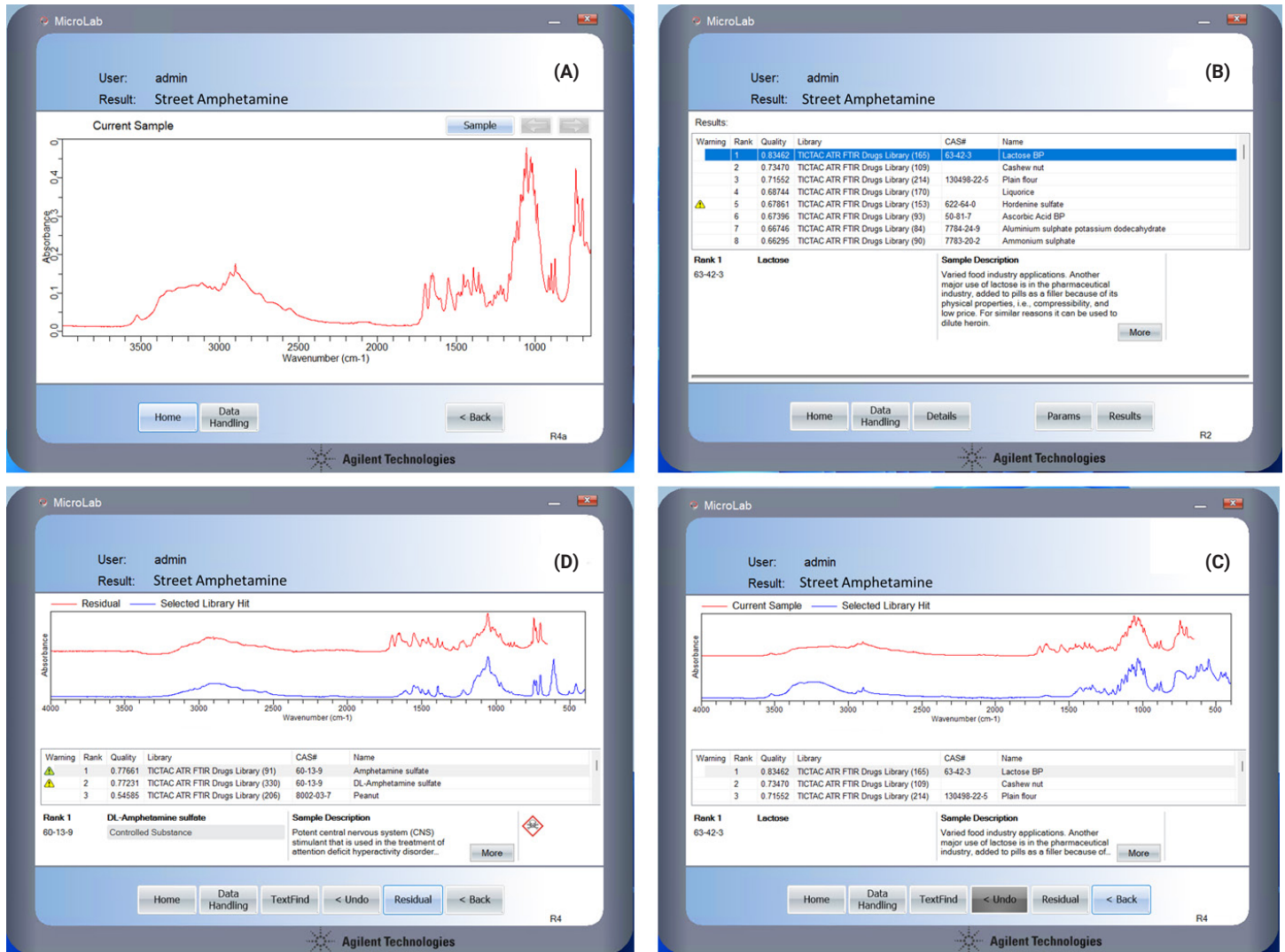
Figure 7. Agilent MicroLab PC software view for a library search of a street sample of amphetamine. Displayed are: (A) street amphetamine FTIR ATR spectrum; (B) ranked library search results for the primary identified compound—lactose BP (HQI% = 83.36%); (C) Details screen for the primary identified compound; and (D) the ranked details of the residual analysis, showing amphetamine sulfate as the residual identified compound (HQI% = 77.66%).
