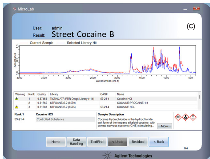
Figure 4. Agilent MicroLab PC software view for a library search of a street sample of cocaine (sample B). Displayed are: (A) cocaine sample B FTIR ATR spectrum; (B) ranked library search results for the primary identified compound—cocaine HCl (HQI% = 87.46%); (C) Details screen for the primary identified compound; and (D) ranked results of the residual analysis, indicating that sodium bicarbonate is the cutting agent (HQI% = 88.31%).
