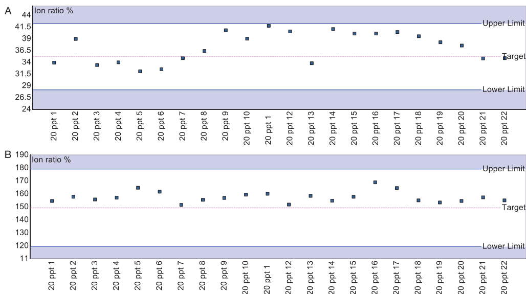
Figure 4. Chromeleon screenshots of the primary confirmation ion ratio of a 20 ng/L standard analyzed over n=132 consecutive injections (over 90 hours of analysis) for 2-MIB (A) and geosmin (B) with ±20% limits indicated. No system maintenance or tuning were performed.
