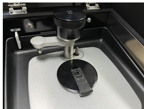
Fig. 2 Specac Arrow accessory on QATR™ 10 ATR accessory
