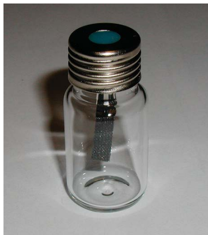
Figure 1. TF-SPME device in 10 mL vial.
