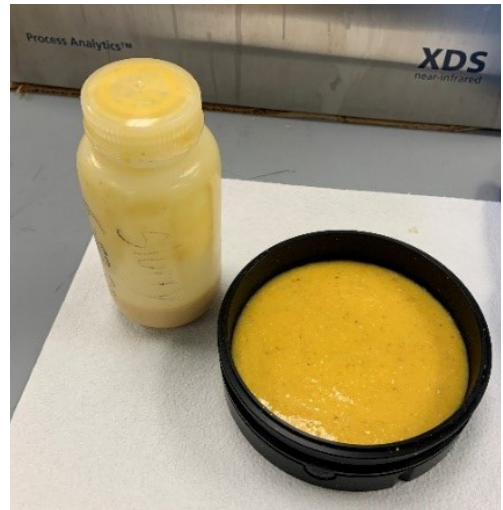
Figure 2. (Left) Ethanol fermentation as measured by NIR spectroscopy. (Right) Sample of corn mash ready for NIRS measurement.
