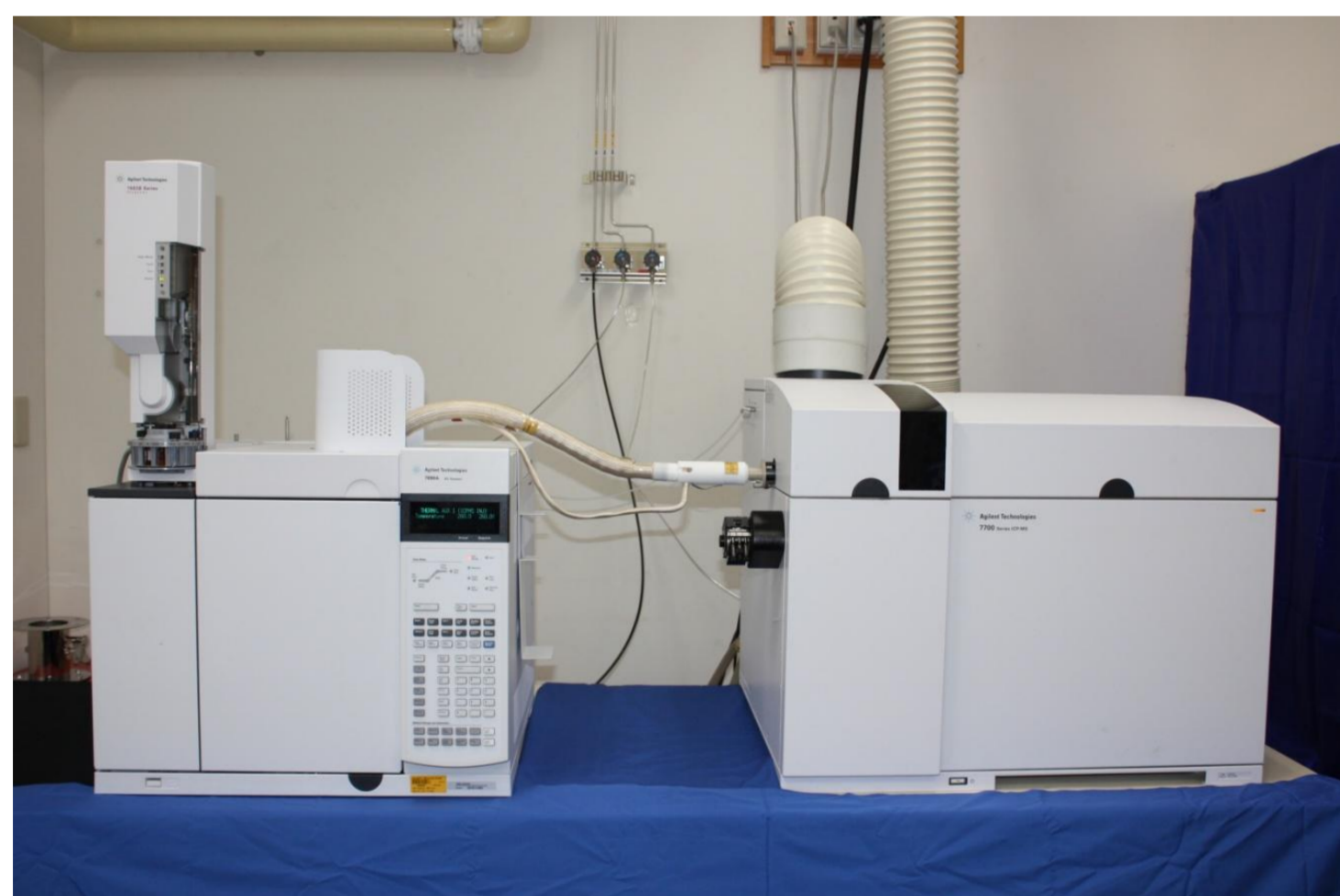
Figure 1. Agilent's ICP-MS coupled to the Agilent's 7890A GC.
